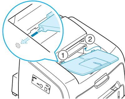
Fold out the extender, if necessary.
