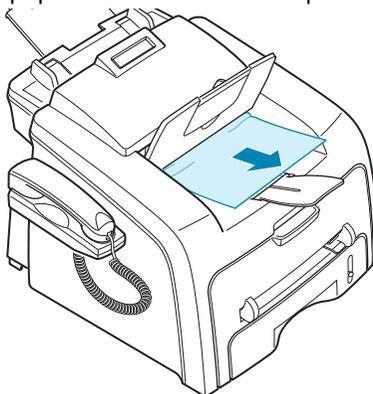
If there is any resistance and the paper does not move when you pull or if you cannot see the paper in the front output tray, continue to step 3.
