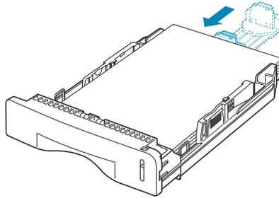
For paper smaller than letter, adjust the paper length guide accordingly.
