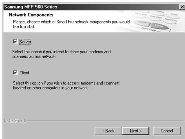
The **Server** option allows you to share a local fax modem and/or a scanner over a LAN. You can control sharing by managing a remote service user. The **Client** option allows you to use Remote Fax or Remote Scan services provided by a SmarThru Server over a LAN. You need to have a client account provided by the server. For details about Remote Fax/Scan Services, refer to the SmarThru User's Guide.
