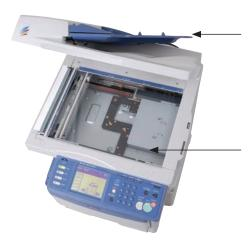
50-sheet reversing automatic document feeder enables the copying, faxing and scanning of multipage, two-sided originals without having to break them into multiple sets. Also supports mixed original copying.
